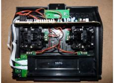
**1.** Open the transmitter, remove the black plastic support frame./
