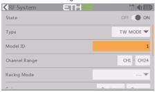
The system assigns the receiver a number for the receiver (Model ID) automatically while creating a new model. (The Model ID can be set from 00 to 63, with the default ID being 1.)
