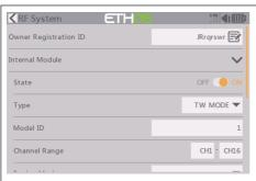
Then turn the state of Internal RF to On. Set the binding mode for the Internal RF module corresponding to the receiver (ACCST D16, ACCESS, TW MODE.etc).
