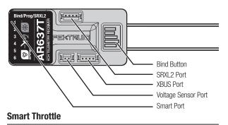
With Smart Technology the normal servo connector delivers the throttle signal to the ESC, plus the ESC can send telemetry data like voltage and current back to the receiver. The AR637T receiver throttle port (Channel 1 port only) will automatically detect when a Smart compatible ESC is connected. ESCs with Smart and IC series connectors can also pass along battery data from compatible Spektrum Smart batteries. Spektrum Avian ESCs are compatible
