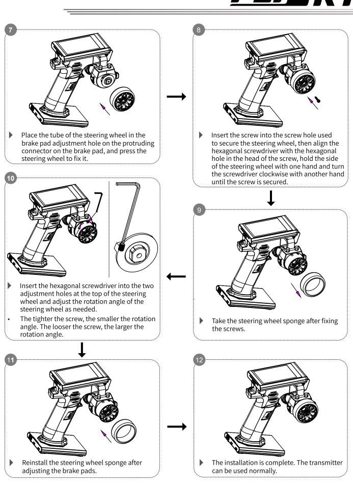
Pay attention to your strength in the process of replacing the brake pads. Remember not to damage accessories. Please refer to the above steps to replace the brake pads, to ensure that the brake pads can be used normally.
