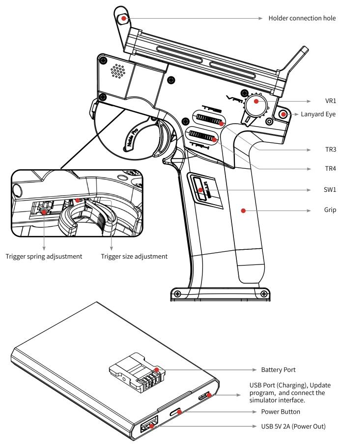
Base power button: Press for a short time to charge the battery at the transmitter handle and to charge external devices. Press 2 seconds to turn off the output of the power supply.
