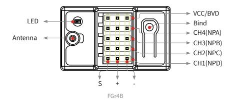
For best signal quality, it is recommended to keep the receiver antenna up and away from metal when installing the FGr8B or FGr4B receivers.
