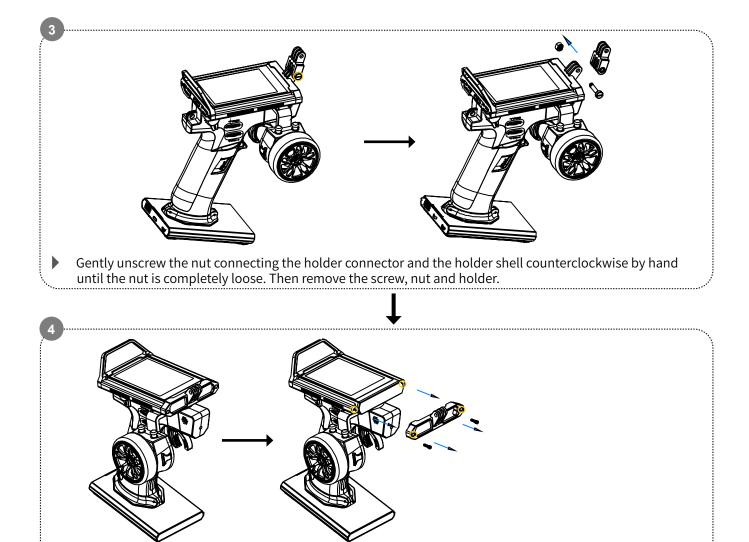
Use a screwdriver to connect the screws on both sides of the top of the screen. Gently turn the screwdriver counterclockwise until the screws on both sides are completely loose. Remove the screws and take off the top holder shell.
