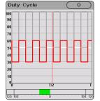
When the period is set to "0", the ratio is 1: 1; When the period is set to "1", the ratio is 1: 2; When the period is set to "-1", the ratio is 2: 1.
